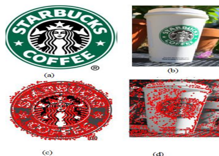
Figure 4.1. Where (a) is the reference logo (b) is the test image (c) Feature points in reference image and (d) is the feature points of test image
